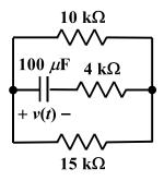
Given v(0) = 100 V, determine v(t) and the power absorbed by the 4 k $\Omega$  resistor for  $t \ge 0$ .
